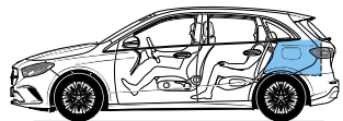
Open luggage compartment behind rear seat, loaded to upper edge of rear seat backrest, volume 420 litres (V 211-2)
