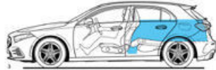
Open luggage compartment behind driver's seat, rear seat backrest folded, loaded to upper edge of driver's backrest, volume 825 litres (V 211-1)
