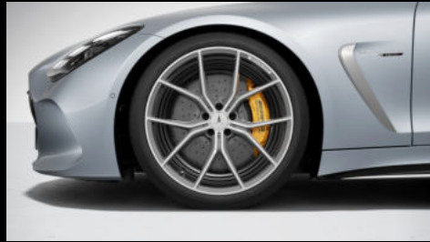
(21-inch) AMG 5-twin-spoke forged wheels aerodynamically optimized, painted in tantalite gray with a high-shine finish (RWI) Optional
