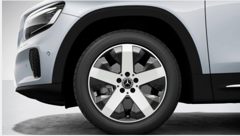
(18-inch) 5-twin-spoke light-alloy wheels (52R) (standard on 200d)
