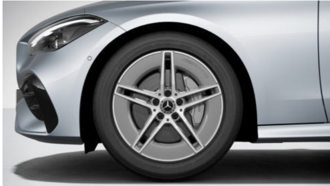
(19-inch) AMG multi-spoke light-alloy wheels, aerodynamically optimised and painted in black with high-sheen rim flange (RVB) □
